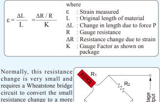
The voltage output of the circuit is given as follows.
