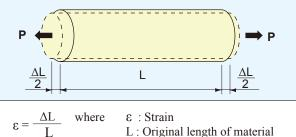
$\Delta L$ : Change in length due to force P Example) when a material of 100mm long deforms by 0.1mm in its length, the resulting strain is as follows.
