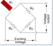
$$e = \frac{R_1 R_3 - R_2 R_4}{(R_1 + R_2)(R_3 + R_4)} E \qquad \begin{array}{c} \text{where} \\ e & : \text{Voltage output} \\ E & : \text{Exciting voltage} \\ R_1 & : \text{Gauge resistance} \\ R_2 \sim R_4 & : \text{Fixed resistance} \end{array}$$
